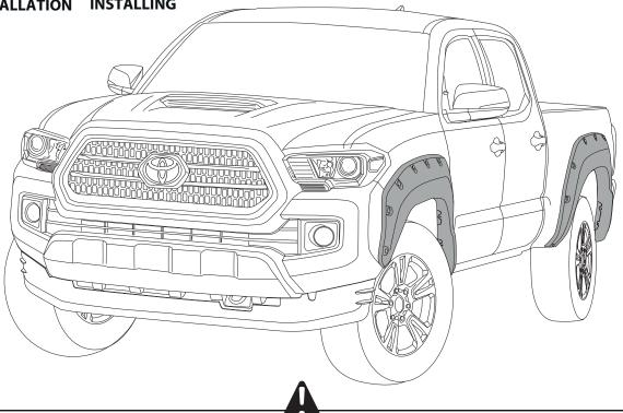
WARNING!! Do not install Hood Scoops or other Body Parts directly Over Wrapped areas. Before installation of the parts, you must leave at least a 1/4" (6mm) perimetral clearance "Free from Vinyl" surrounding the part, before Part installation.
