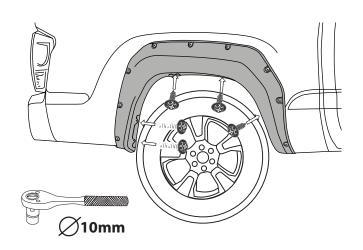
23 APPLY LOCTITE THREADLOCKER TO SUPER-BOLTS THREAD
